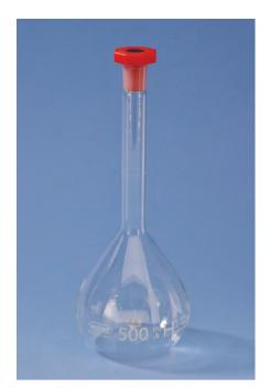
Flasks, Volumetric, Class A, clear glass
